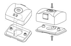
Figure 12. Connecting the stimulator to the electrode pad
